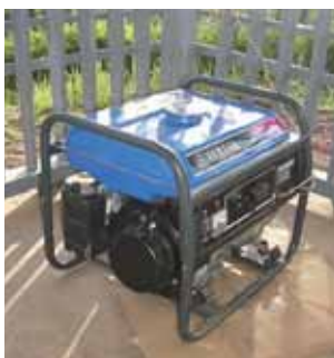
Fig. 33. This generator will provide about two hours of electricity at night. It often broke down because of sand and water contamination of the gasoline.
