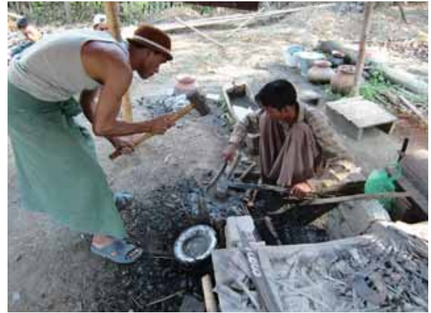
Fig. 2. Shaping the heated iron. Saw. February 18, 2009.
