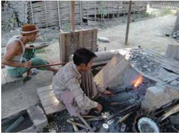
Fig. 1. Sending air with a bellows. Saw. February 18, 2009.
